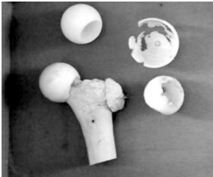
Figure 4: Charnley PTFE double cup implant, c. 1960.
