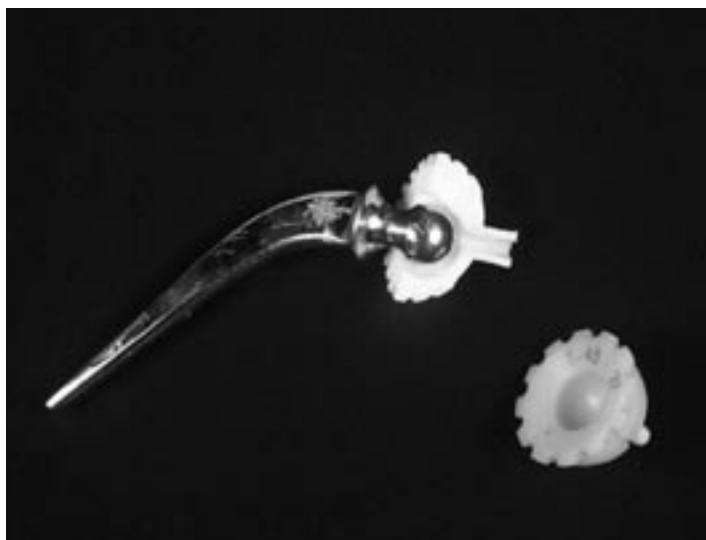
Figure 15: The Charnley low-friction arthroplasty in use from November 1962, having a thick socket of UHMWPE with deep external serrations and a small femoral-head on the flat-back prosthesis.
